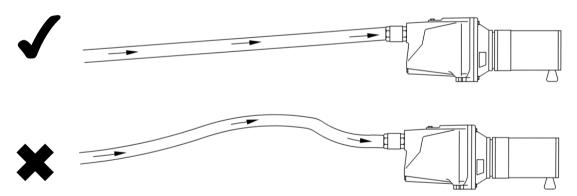
6. The **inlet line** to the pump should be as short and straight as possible, with a bore at least as large as the nominal bore of the pump inlet port. Use rigid or reinforced pipe that will not deform or collapse under suction conditions. The inlet pipe should be angled below the horizontal, to prevent entrapment of air and loss of prime when running.
